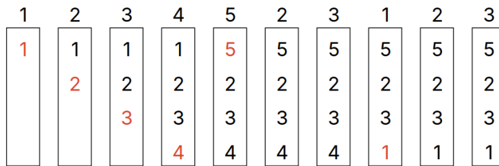
Figure 1: Clock replacement example. 6 total page faults.
