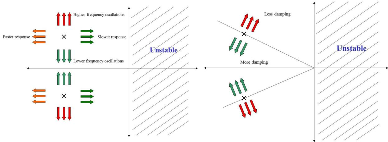
Figure 4: Response based on pole location.
