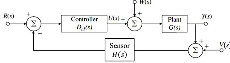
Figure 6: Closed-loop controller with disturbances.
