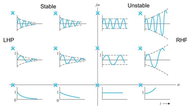
Figure 1: Behaviour of a system according to its poles.
