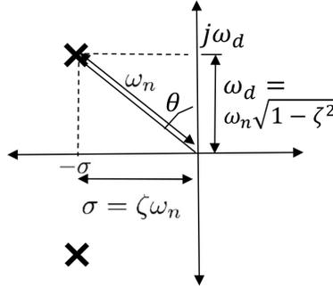
Figure 3: Pole locations for underdamped system.
