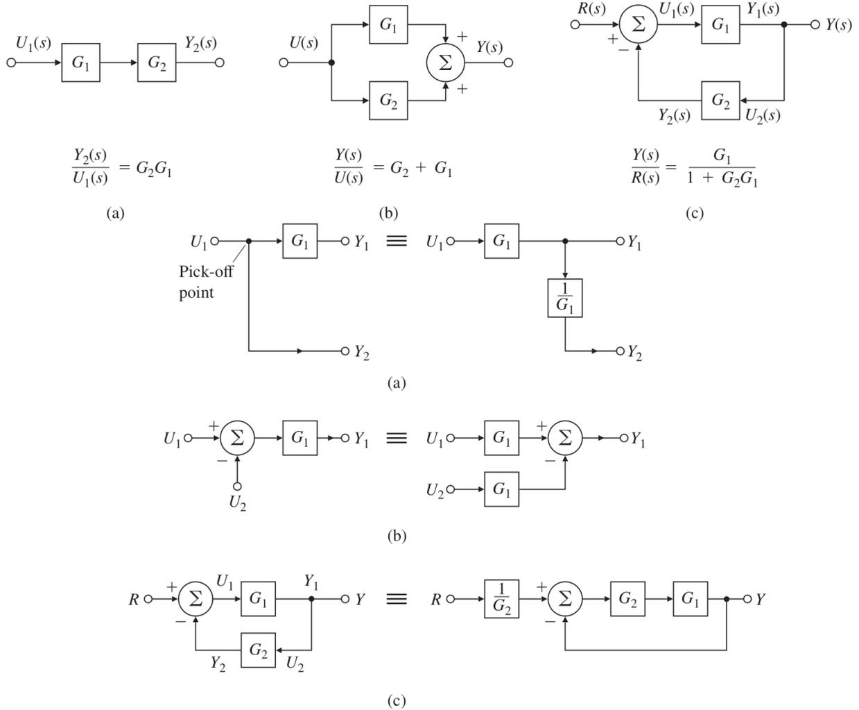
Figure 5: Block diagram reduction rules.
