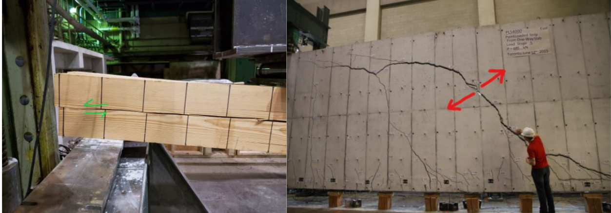
Figure 3: Failure due to shear stresses
