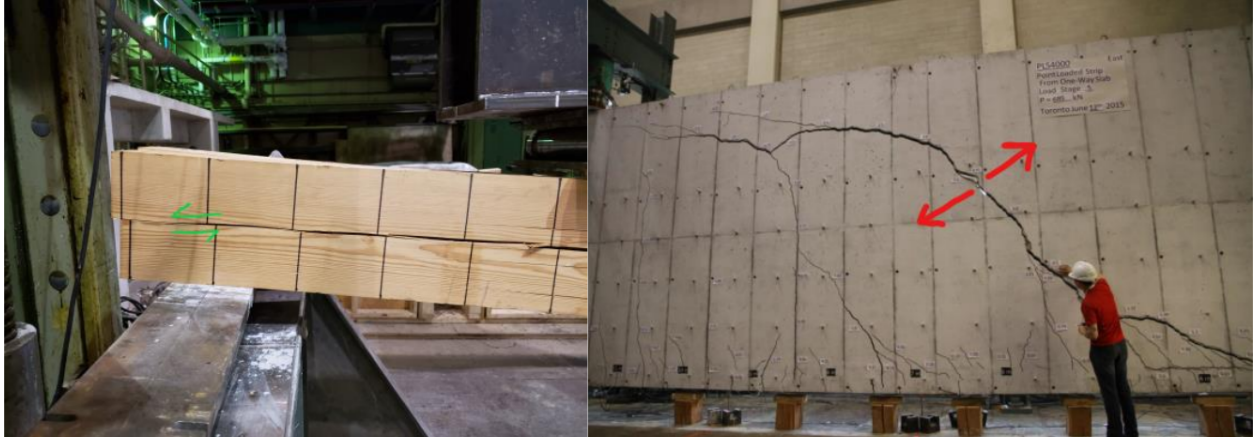
Figure 48: Failure due to shear stresses
